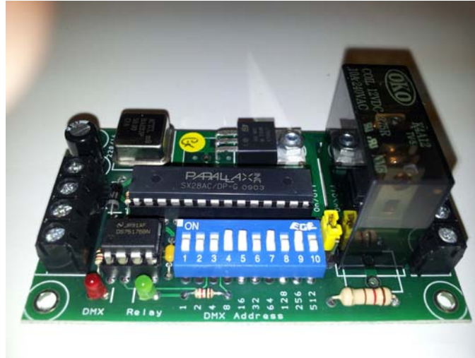
Slika 4. DMX512 prekidač 10A, Milford Instruments Limited UK
